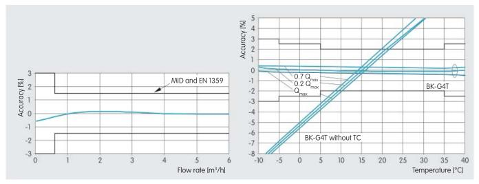
With calibration error limits at test room temperature
